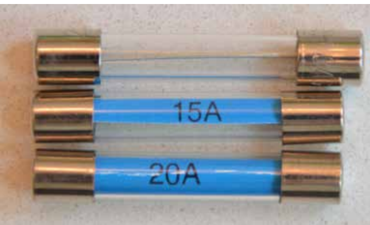
Upper fuse is a longer AGC-type with incorrect rating. Lower fuses are OEM Lucas type
