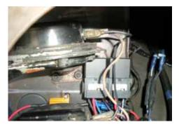
Michael placed the relays controlling his headlights adjacent to the horns, hidden behind the left outer headlight. Another part of Michael's electrical project was to add a relay to the relay panel so that the headlights only have power when the key is turned on. The gold resistor visible just above the lower horn is for daytime running lights.
